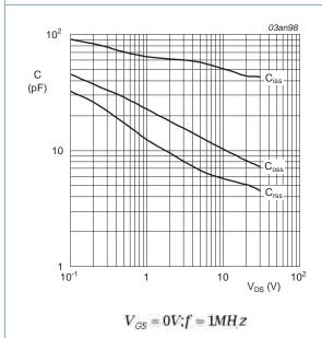
Fig 11. Input, output and reverse transfer capacitances as a function of drain-source voltage; typical
