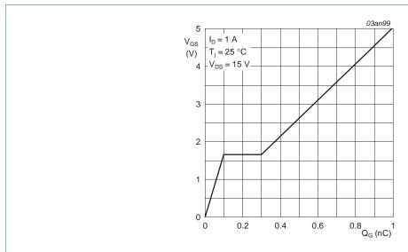
Fig 13. Gate-source voltage as a function of gate charge; typical values
