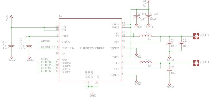
Figure 7. Minimum component schematic of IDTP9122.
