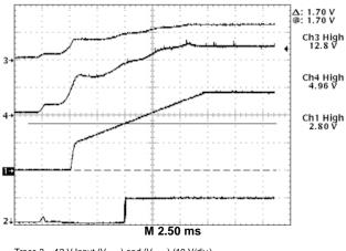
$\label{eq:constraint} \begin{array}{l} \mbox{Trace 3 - 12 V Input (V_{CC1}) and (V_{CC2}) (10 \mbox{V/div.}) \\ \mbox{Trace 4- 5.0 V Input (2.0 \mbox{V/div.}) } \\ \mbox{Trace 1- Regulator Output Voltage (1.0 \mbox{V/div.}) } \\ \mbox{Trace 2- Power Good Signal (2.0 \mbox{V/div.}) } \end{array}$
