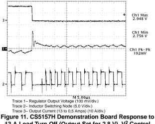
13 A Load Turn Off (Output Set for 2.8 V). V<sup>2</sup> Control Topology Immediately Connects Inductor to Ground, Providing 0% Duty Cycle. Regulation is Achieved in Less Than 10 μs
