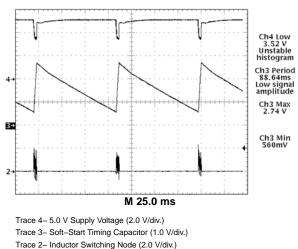
Figure 12. CS5157H Demonstration Board Hiccup Mode Short Circuit Protection. Gate Pulses are
