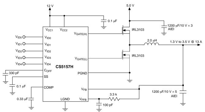
Figure 1. Application Diagram, Switching Power Supply for Core Logic – Pentium<sup>®</sup> II Processor
