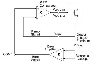
Figure 3. V<sup>2</sup> Control Diagram
