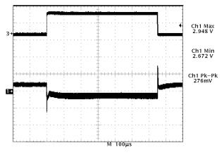
Trace 1– Regulator Output Voltage (100 mV/div.) Trace 2– Regulator Output Voltage (10 A/div.)
