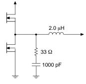
Figure 20. Filter Components
