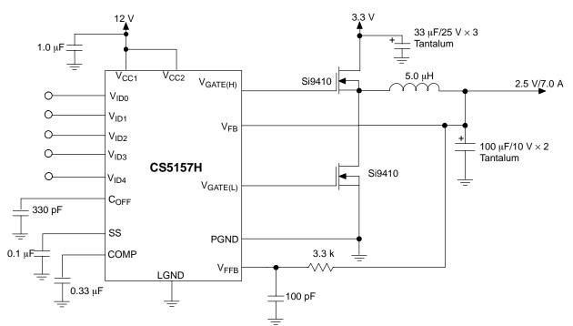
Figure 24. Additional Application Diagram, 3.3 V to 2.5 V/7.0 A Converter with 12 V Bias
