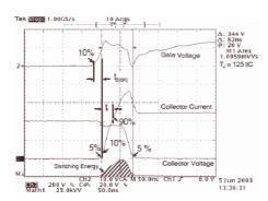
Figure 18, Turn-on Switching Waveforms and Definitions
