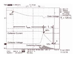
Figure 19, Turn-off Switching Waveforms and Definitions
