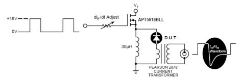
Figure 9, Diode Test Circuit
