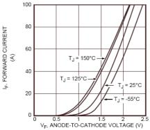
Figure 2. Forward Current vs. Forward Voltage
