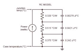
FIGURE 1b, TRANSIENT THERMAL IMPEDANCE MODEL
