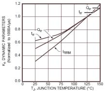
Figure 6. Dynamic Parameters vs. Junction Temperature
