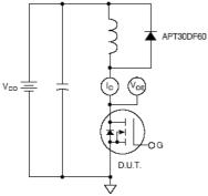
Figure 20, Inductive Switching Test Circuit
