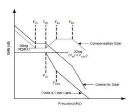
Figure 15. Converter Gain and Frequency
