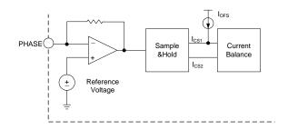
Figure 2. R<sub>DS(ON)</sub> Current Sensing Scheme
