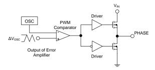
Figure 13. The PWM Modulator
