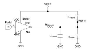
Figure 6. PWM-VID Analog Circuit Diagram
