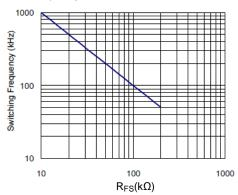
Figure 1. Switching Frequency vs. R<sub>FS</sub>
