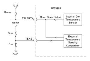
Figure 4. Thermal Alert and Temperature Sense
