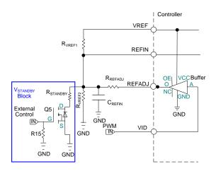
Figure 7. Integrated Buffer Circuit
