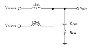
Figure 11. The Output LC Filter
