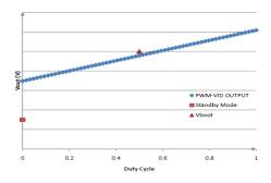
Figure 9. Illustration for Standby Mode and Adjustable V<sub>BOOT</sub> Setting
