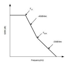
Figure 12. Frequency Response of the LC Filters
