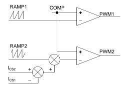
Figure 3. Current Balance Scheme of AP3598A
